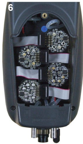
Connection of the sensor ribbon cable
